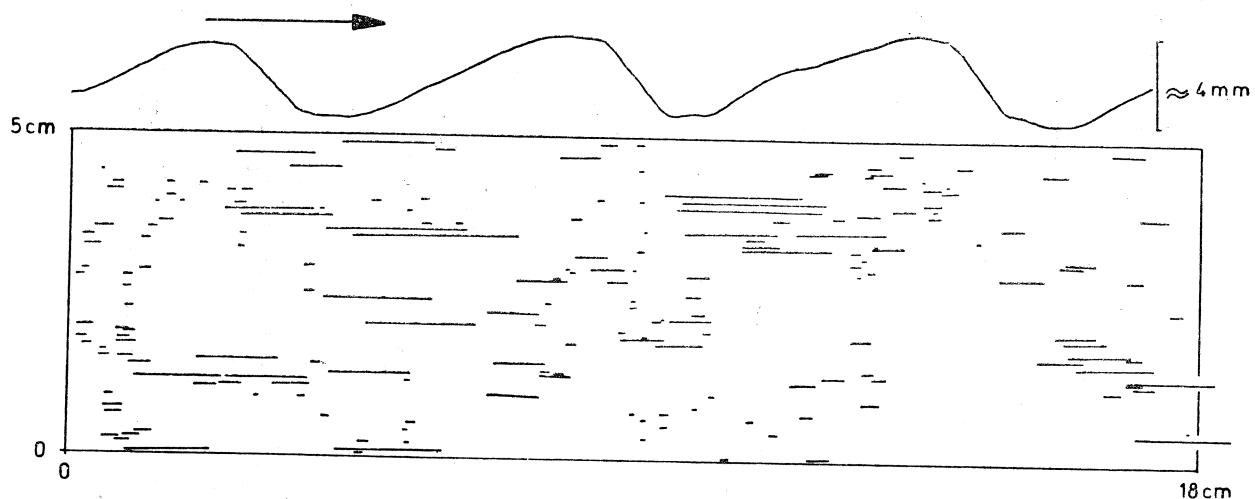
Fig. 5. Grain paths measured with the time paralaxe method. Area of observation is indicated on fig. 2. Profile of ripples represents situation in the cetrum of the rectangle
