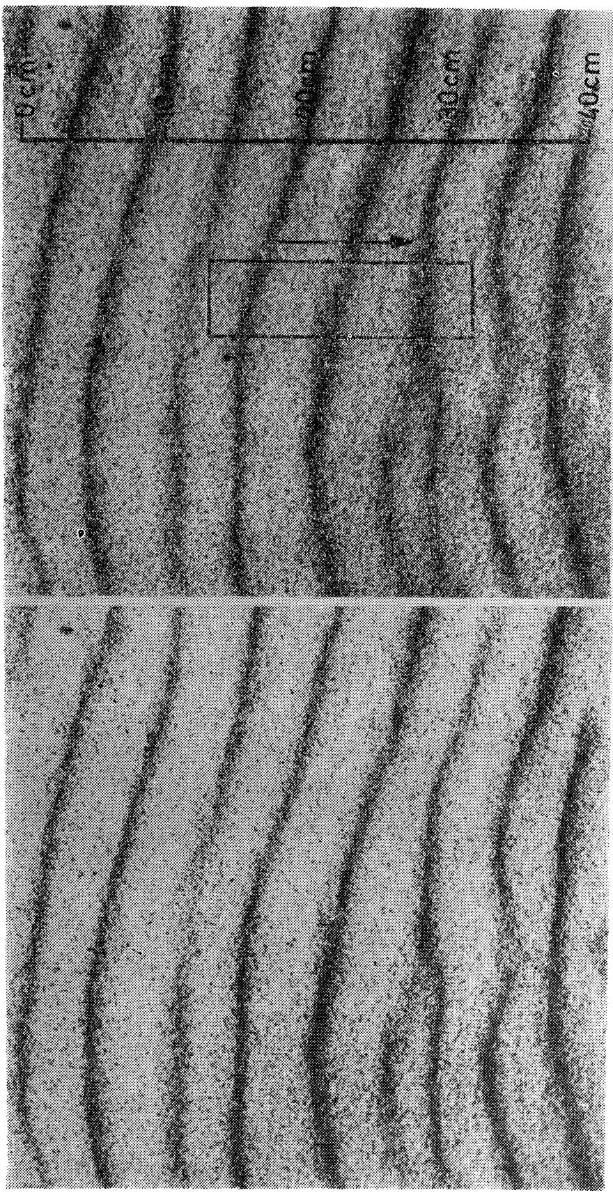
Fig. 2. Stereopair of ripples developed on the tunnel bed
