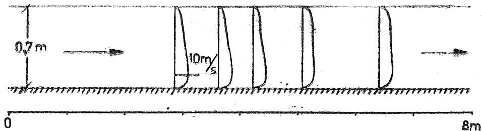
Fig. 1. Velocity distribution inside the tunnel
