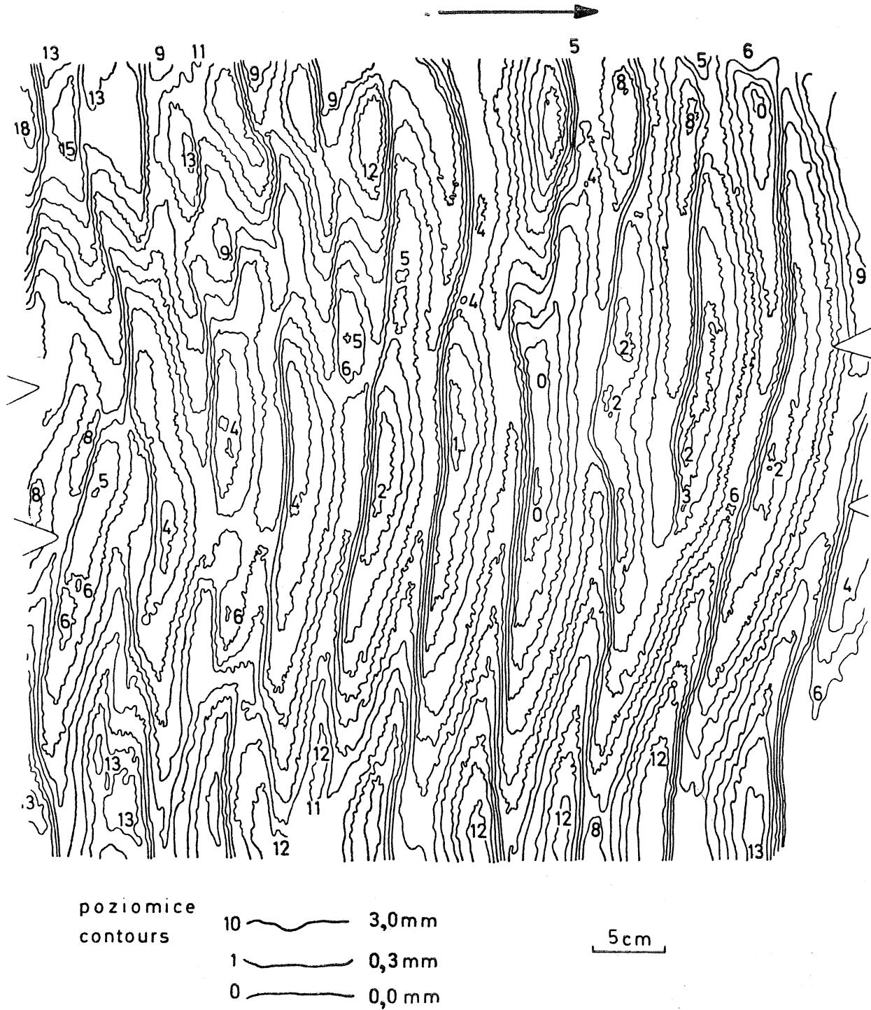
Fig. 4. Countour map of ripples developed after 180' from start
