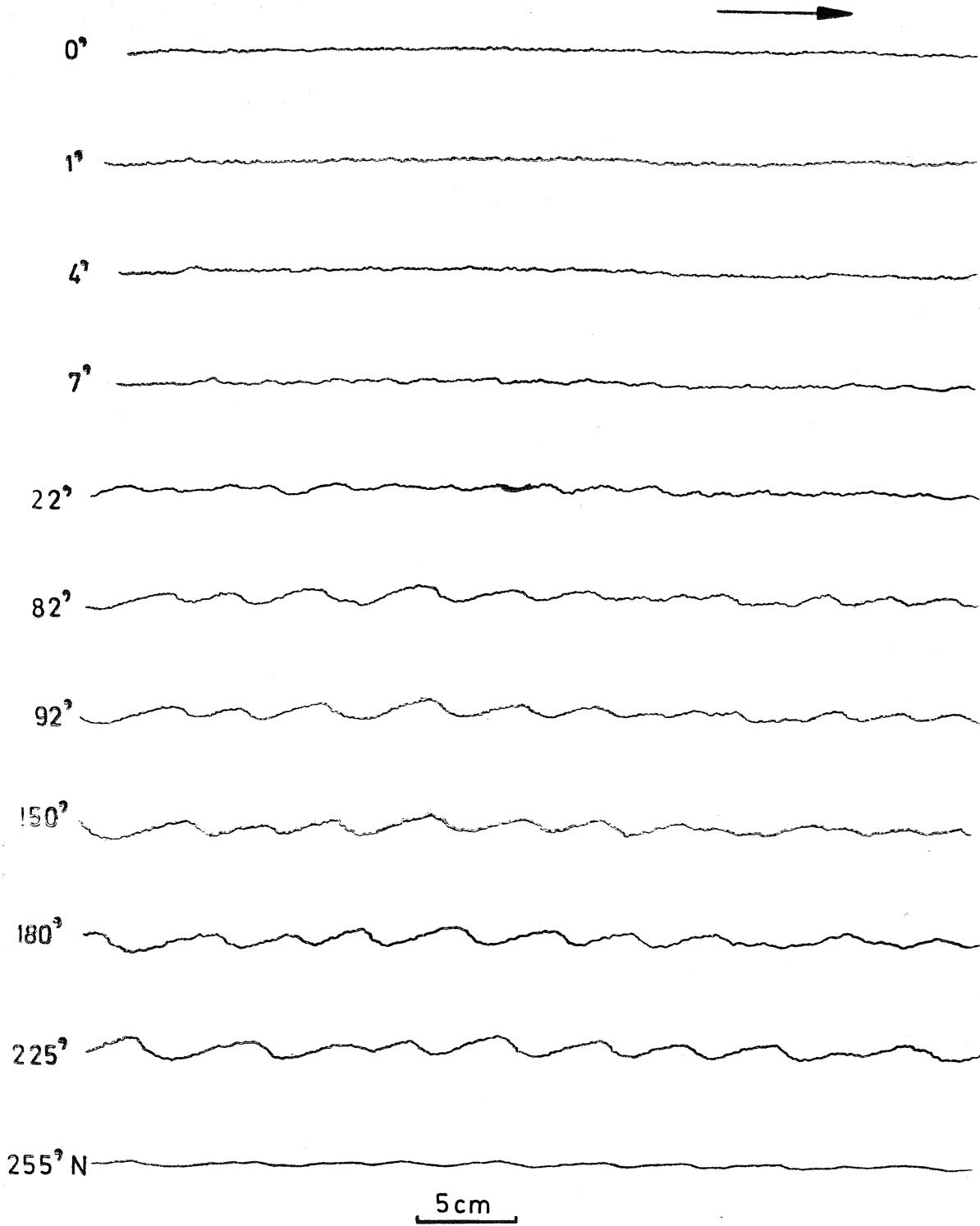
Fig. 3. Profiles of the tunnel bed during development of ripples Numbers 1'—225'
