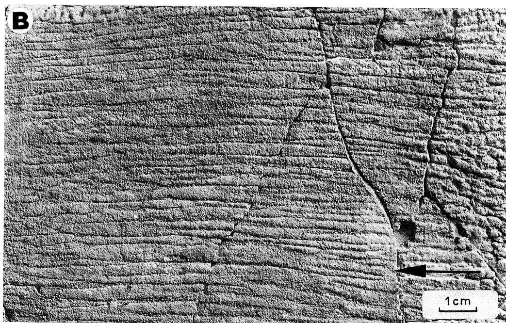
Plate 32 (A) Closely spaced moulds of l-ridges. Oligocene Krosno Beds, Rudawka Rymanowska. (B) Closely spaced moulds of l-ridges. Base of artificial turbidite (after Dżułyński, 1965)
