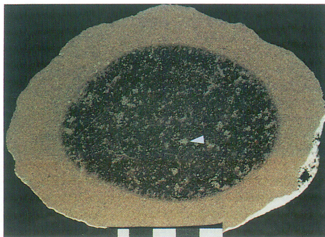
Fig. 4. Polished slab of an exotic organodetrinitic Lithothamnium limestone of calcarenitic type. Irregular outer surface is visible along with central cherty core which reflects the shape of the surface and contain equally-spaced enclaves of unsilicified rock (arrowed). Site 4 (Kosztowa); bar scale in centimetres
