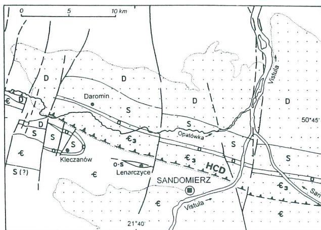
**Fig. 1.** Geological map of the eastern part of the Holy Cross Mountains (After Pożaryski and Tomczyk, 1993, generalized). HCD – Holy Cross Disclocation; € – Cambrian; €<sub>3</sub> – Upper Cambrian; O – Ordovician; S – Silurian; D – Devonian; uninterrupted and interrupted thick lines – faults; dotted lines and dotted area – extent of Tertiary of the Opatówka River; big black circle – bore-hole
