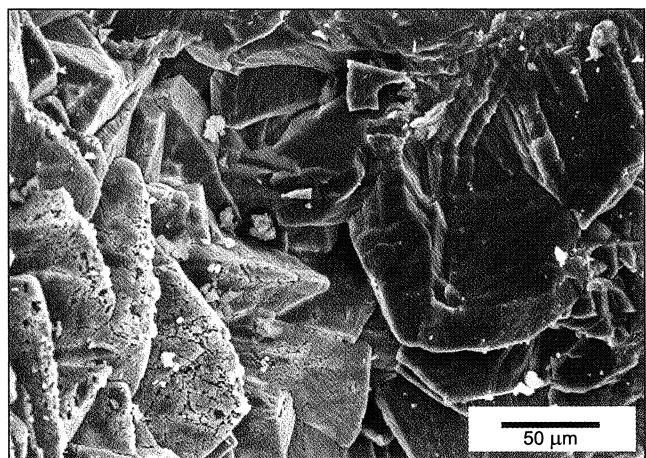
**Fig. 12.** Sparitic cement of moss travertine; SEM image
