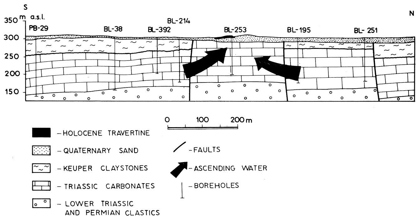
Fig. 5. Geological cross section of the study area
