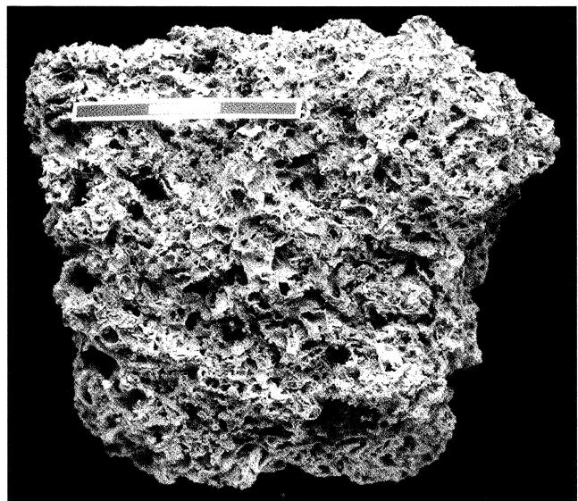
Fig. 7. Moss travertine with primary porosity, scale bar 3 cm
