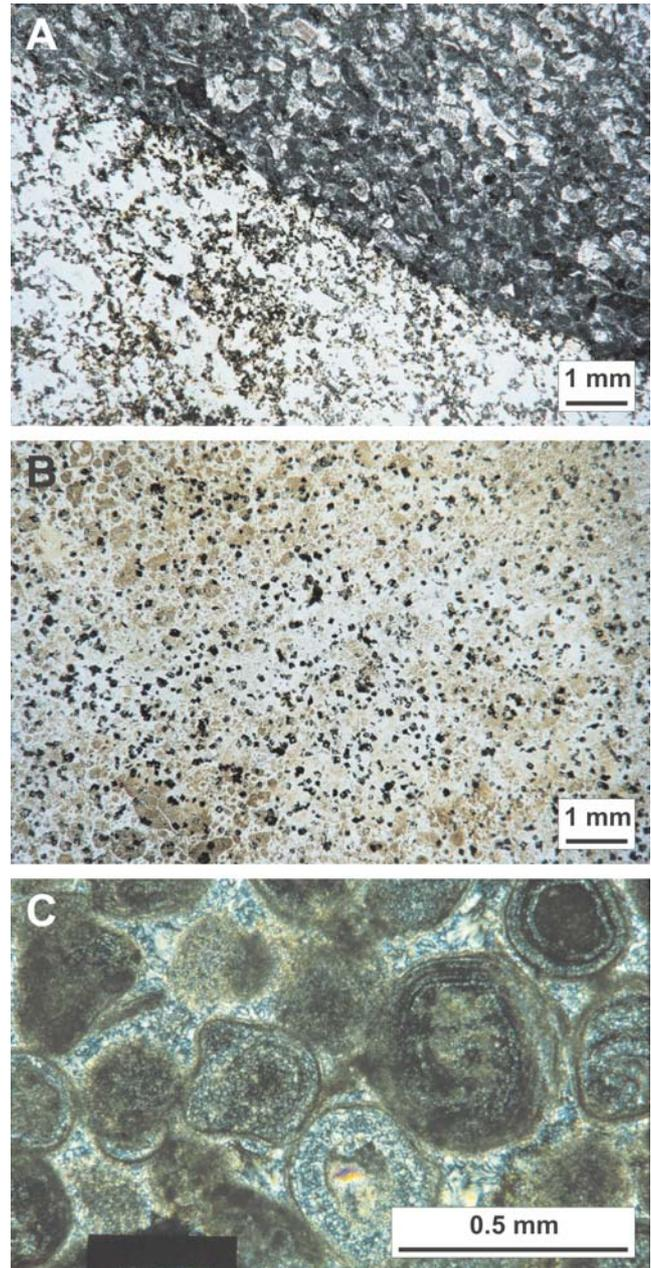
**Fig. 5.** A – Two parts: contaminated zone dominated by carbonate (dark), and a zone dominated by silica (light). Sponge spicules visible. Łukowa eds; Wolica; B – The micro-quartzitic and micro-chalcedonic chert with silicified pellets and carbonate rhombohedrons decaying in the centres. Karchowice beds, Tarnów Opolski; C – Silicified oncoidal limestone. Oncoids silicified to a different degree. Chalcedonic matrix. Gogolin beds, Płaza
