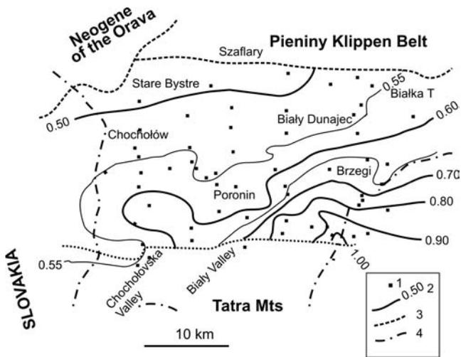
**Fig. 7.** Sketch-map of changes in mean random reflectance of vitrinite (colotelinite) of coal and coaly matter from the Podhale Flysch. 1 – samples; 2 – isolines of total random reflectivity ( $R^0I + R^0II$ ) – spacing 0.05% ( $R^0I + R^0II$ ); 3 – border of the Tatra Mts and the Pieniny Klippen Belt; 4 – state boundary
