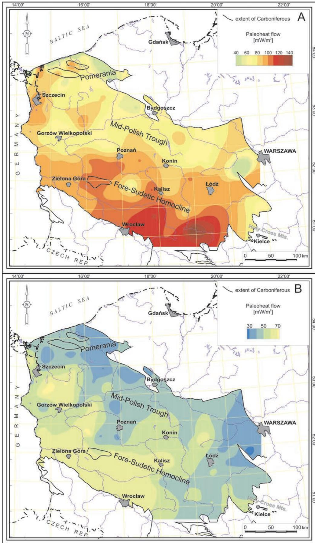
**Fig. 10.** Palaeo-heat flow: Variscan (A), Cretaceous (B)
