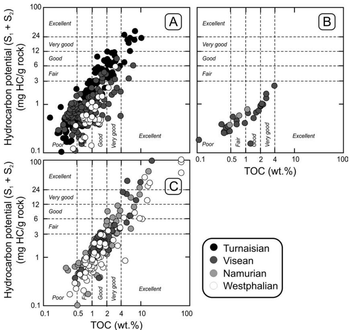
**Fig. 5.** Petroleum source quality diagram for Carboniferous strata in (A) Pomerania, (B) Fore-Sudetic Homocline and (C) Masovia-Lublin area. Classification after Hunt (1979) and Peters and Cassa (2002). Data modified after Bachleda-Curuś *et al.* (1996), Burzewski *et al.* (1998), Matyasik (1998), Nowak (2003), Kotarba *et al.* (1999, 2004, 2005), Kosakowski *et al.* (2006), Pletsch *et al.* (2010), and Poprawa (2010)
